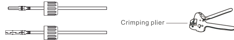
▲ Figure 4.12 Crimp the contact pin to the wire
